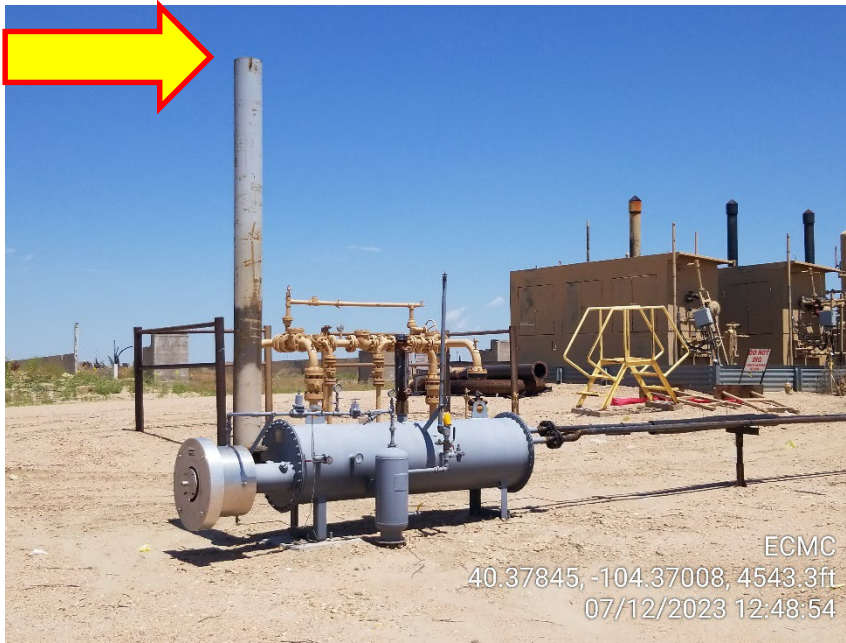
Photo 5 – Line Heater – Missing Bird Protector
