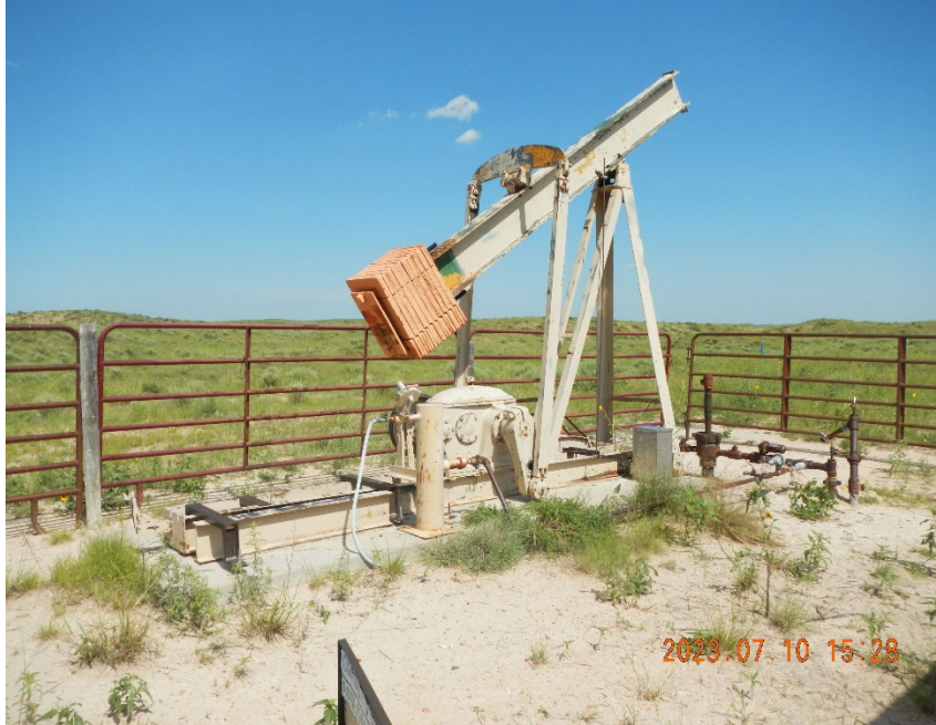
3. View of Pump Jack with motor removed.
