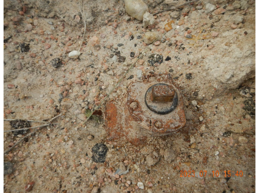
6. Surface casing valve open to atmosphere.
