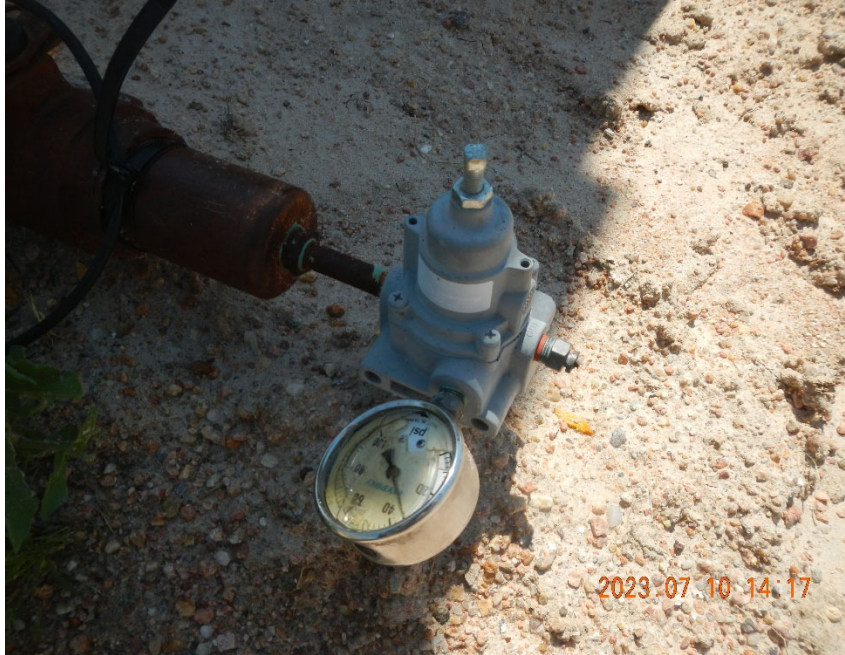
7. Venting Regulator at wellhead.
