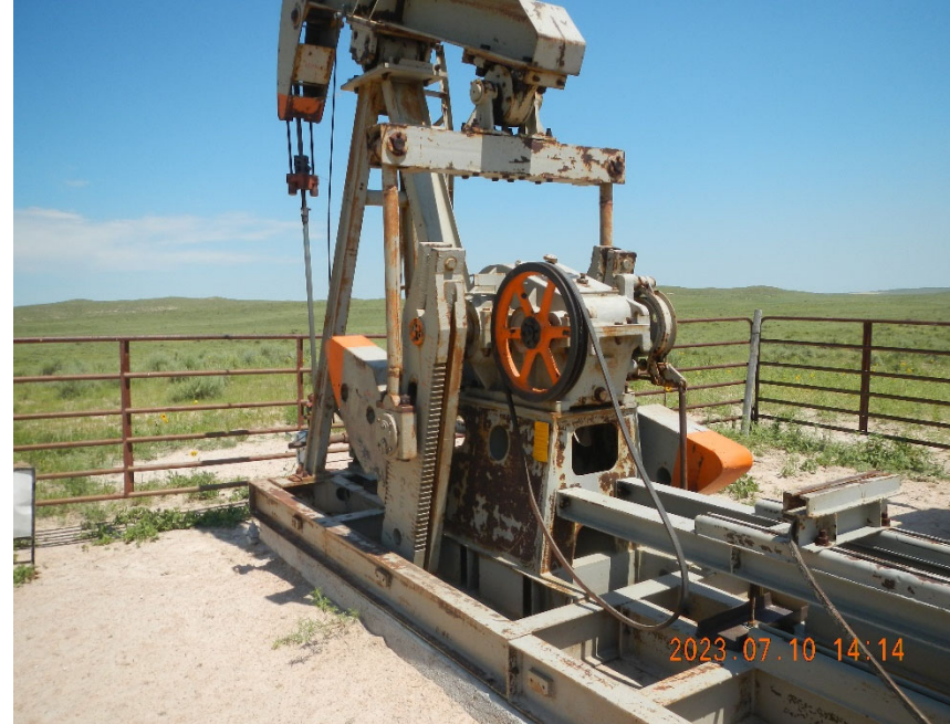
4. Motor removed from Pump Jack.
