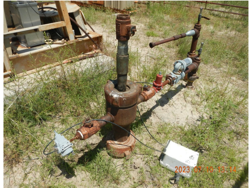
2. View of wellhead. Casing valve closed.
