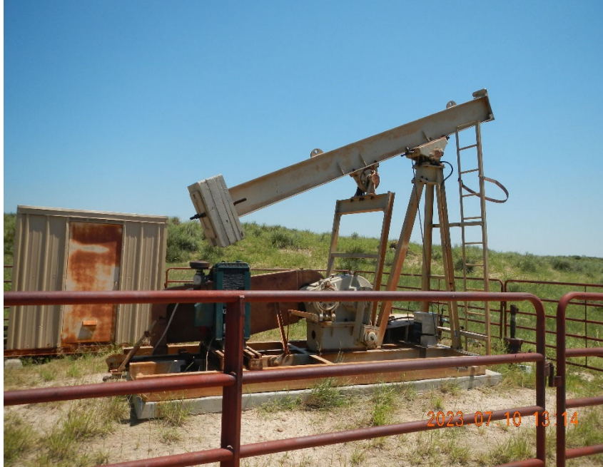
3. Pump Jack and Meter/Separator Shed.
