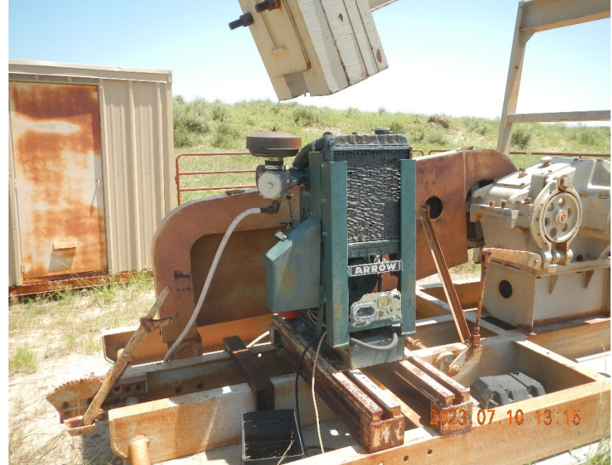
4. Pump Jack Prime Mover Gas Motor.
