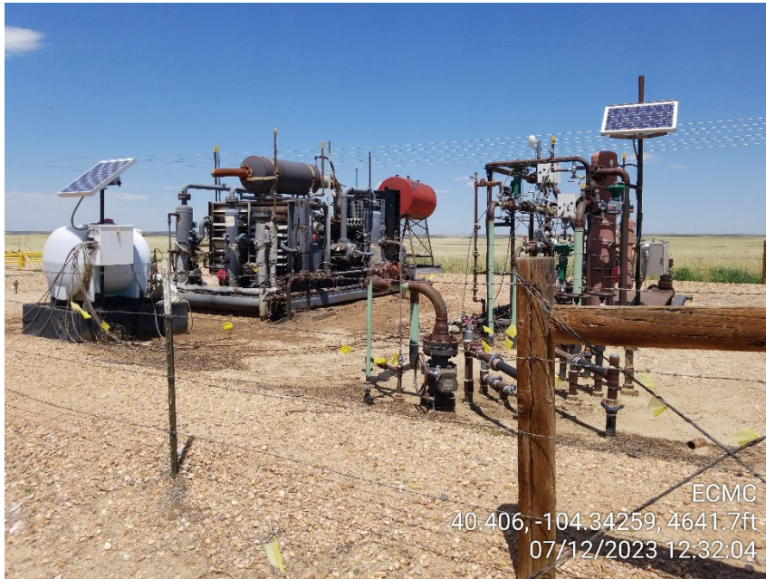
Photo 7 – Compressor and Gas Lift Injection Meters
