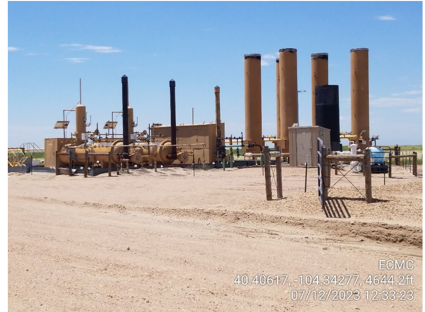
Photo 12 – ECDs and Separators
