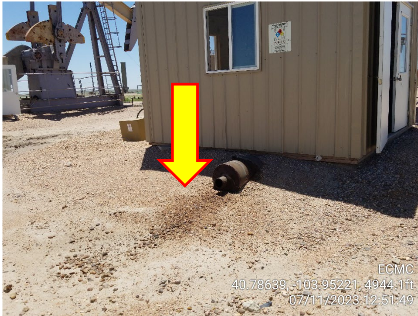
Photo 5 – 02-0214H Exhaust – Stained Soil
