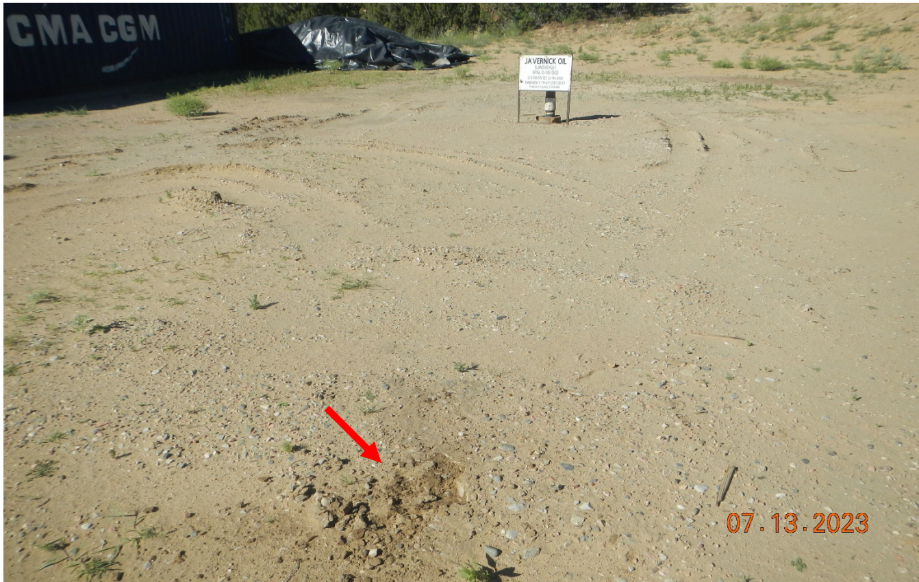
Photo 19. Facing southwest toward the wellsite. Sign is posted at the wellhead. The area at the red arrow has hardened oil stained soil from where the drilling rig was parked. Areas of contaminated soil must be cleaned up.
