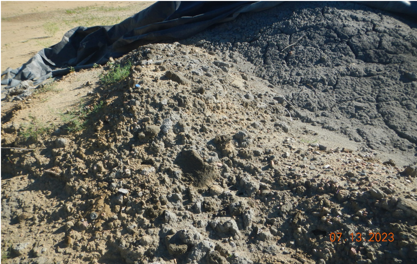
Photo 17. There is also oily soils that are mixed in with the drill cuttings. This was not previously observed and may have come from clean up of the oily soils at the tank battery. The E&P waste are not properly stored and contained.
