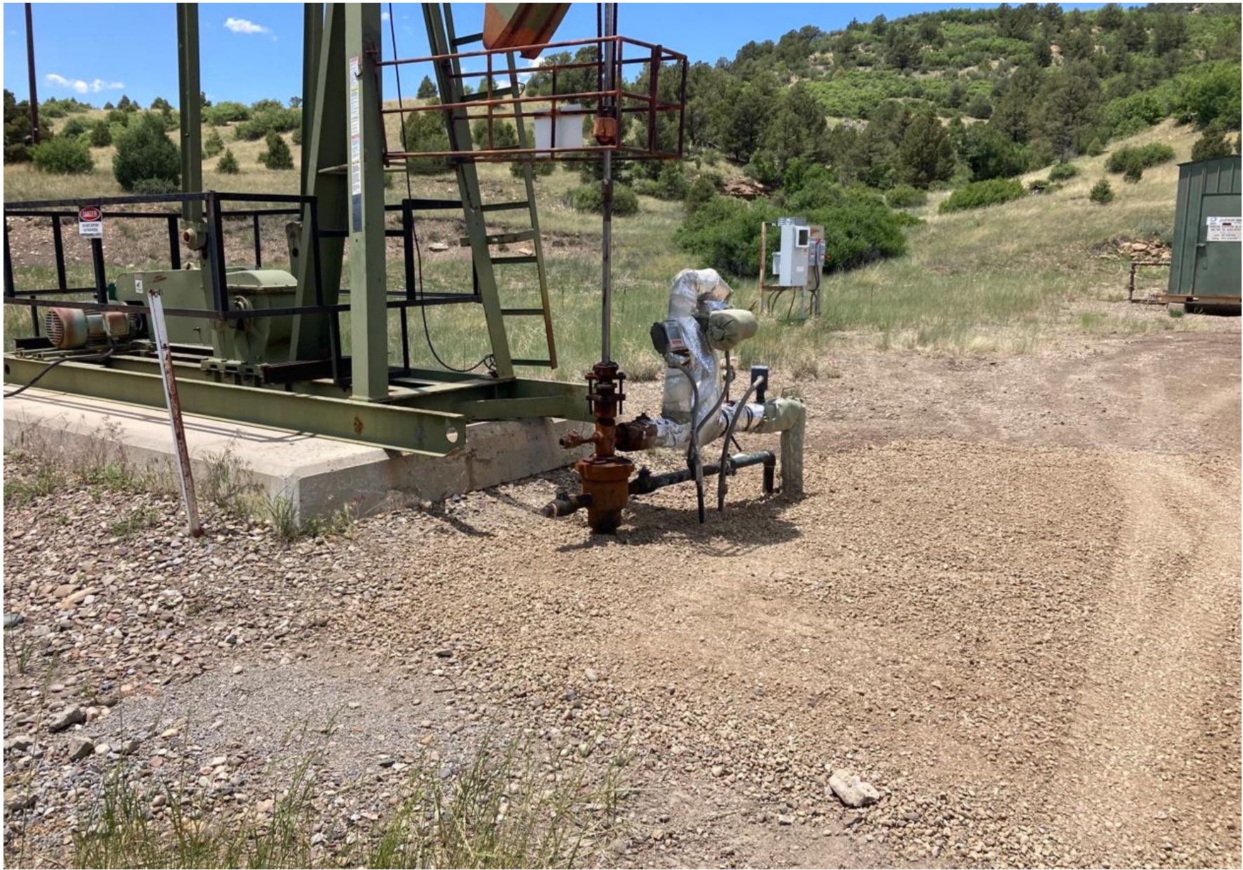
PHOTO 1: THE LEAKING PACKING AS BEEN FIXED AND MAINTENANCE HAS BEEN PERFORMED TO OPERATING EQUIPMENT. THE SPILL WAS CONTROLLED IMMEDIATELY UPON CONTACT FROM COGCC INSPECTOR. ALL STANDING LIQUIDS AND CONTAMINATED SOILS WERE REMOVED FROM LOCATION AND PROPERLY DISPOSED OF. THE SELF INSPECTION PROCESS HAS BEEN REVIEWED.
