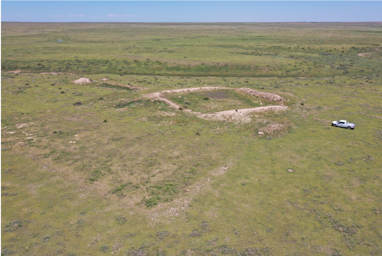
Photo 1. Drone aerial photo facing northeast toward the abandoned well location. The pits were have not been backfilled and reclaimed
