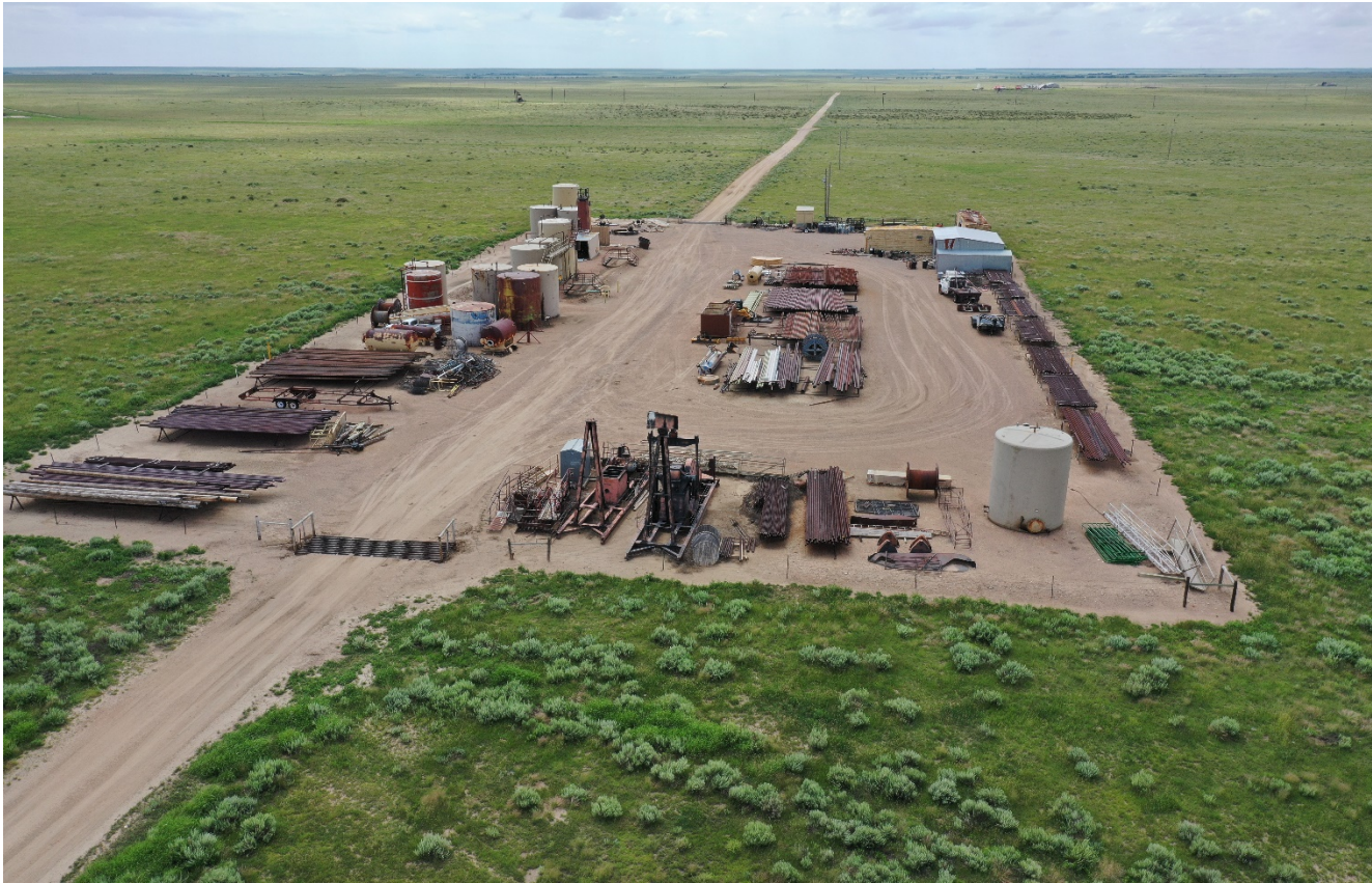
Photo 1. Drone aerial photo facing west toward the PYLES offsite tank battery and storage yard. The use of this location as a storage yard is prohibited per the rules. All unused equipment and supplies must be removed and interim reclamation must be performed.
