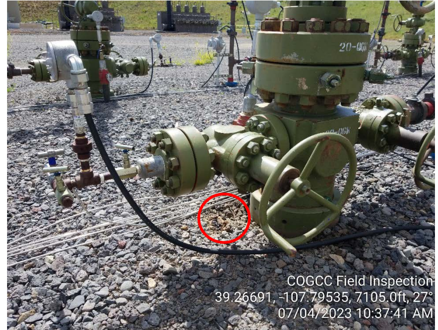
Photo #6 – Localized accumulation of oily waste beneath 20-06W wellhead.
