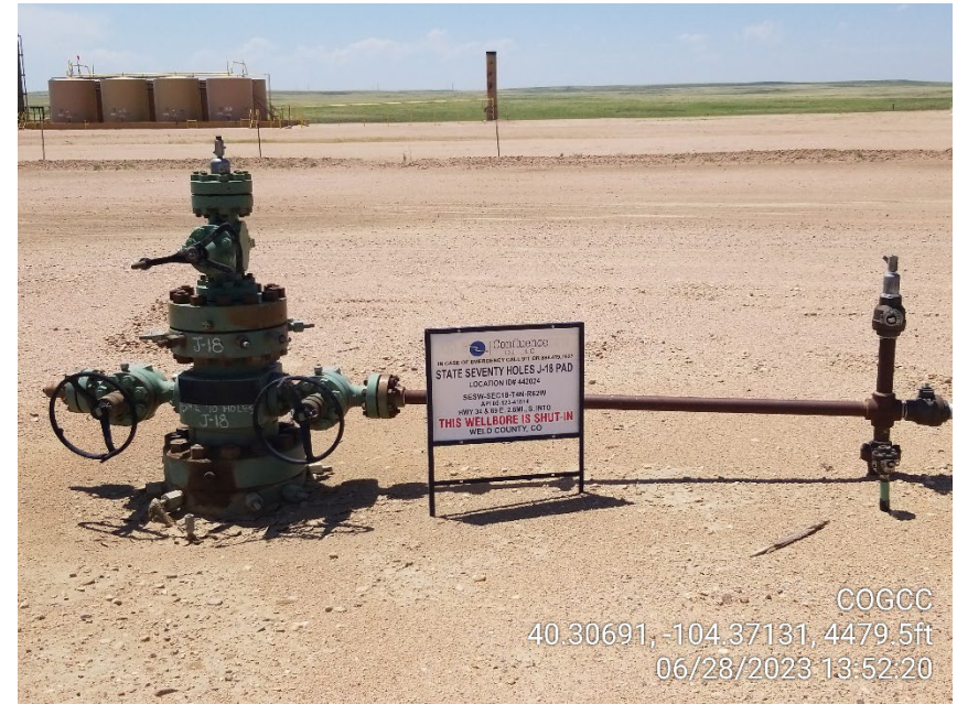
Photo 10 – State Seventy Holes J-18 TA Wellhead
