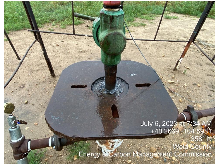
Mechanical Conditions “leaking packing”
