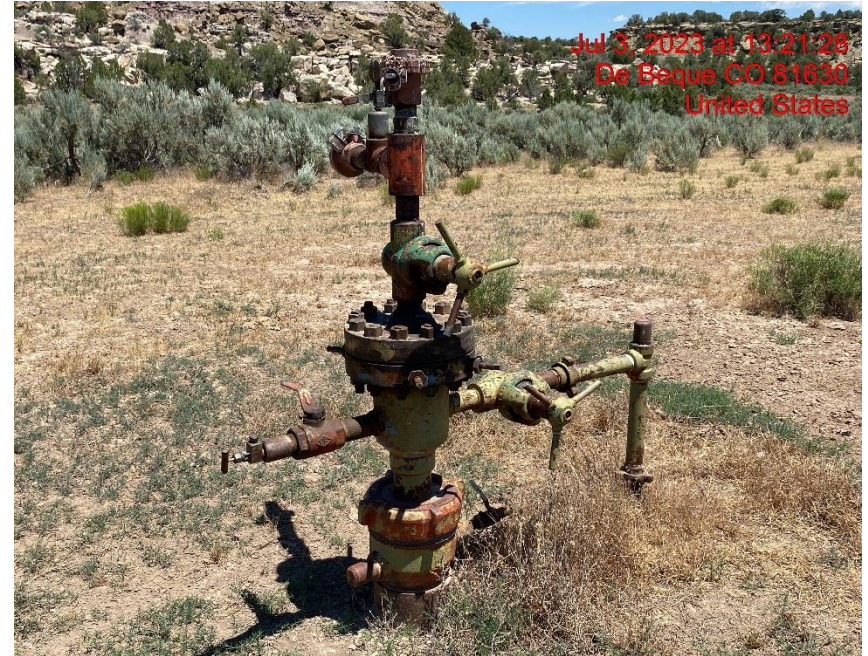
Wellhead/Missing Sign – Photo #04970
