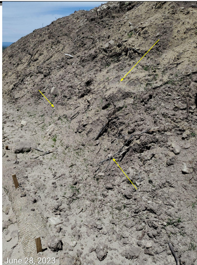
Photo 23: See comments under photo 21. Areas above top arrow include residual hydromulch, however, the fine soils (light colored soils) appear to have also been blown onto these areas of the soil stockpile as well.
