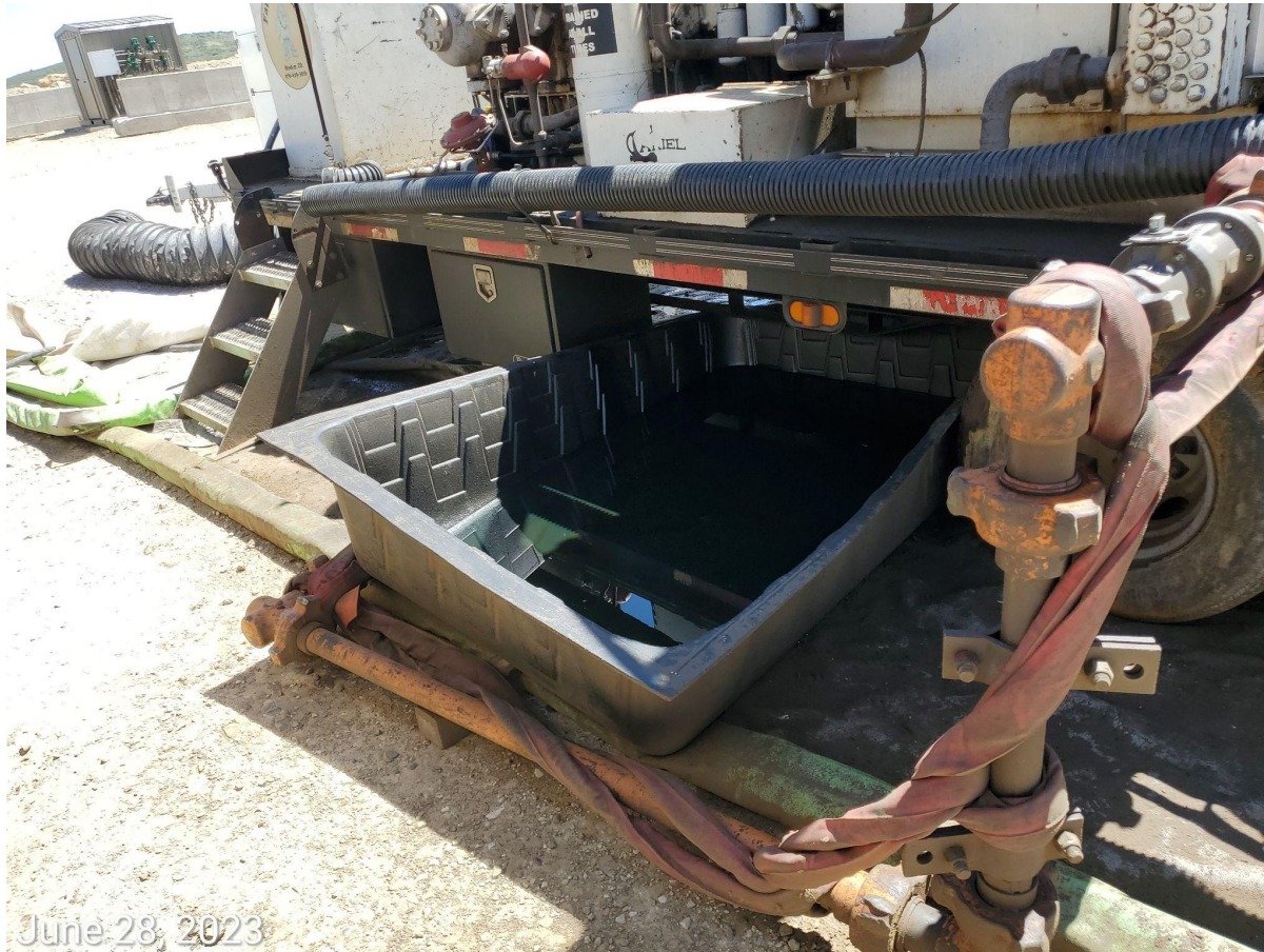
Photo 14: Containment BMP at the Gas Lift equipment with fluids.
