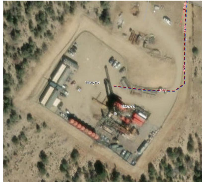
Measuring approx. 3.51 acres disturbed, an average of 6-inches of topsoil removed at the start of wellsite construction resulted in over 2800 cu. yds of topsoil stored at the location. No additional topsoil imported to the location as amounts satisfies estimated amounts. Topsoil areas are labeled with signage to designate it as separate from the normal operating pad. Areas are stabilized with hydromulched seed.
