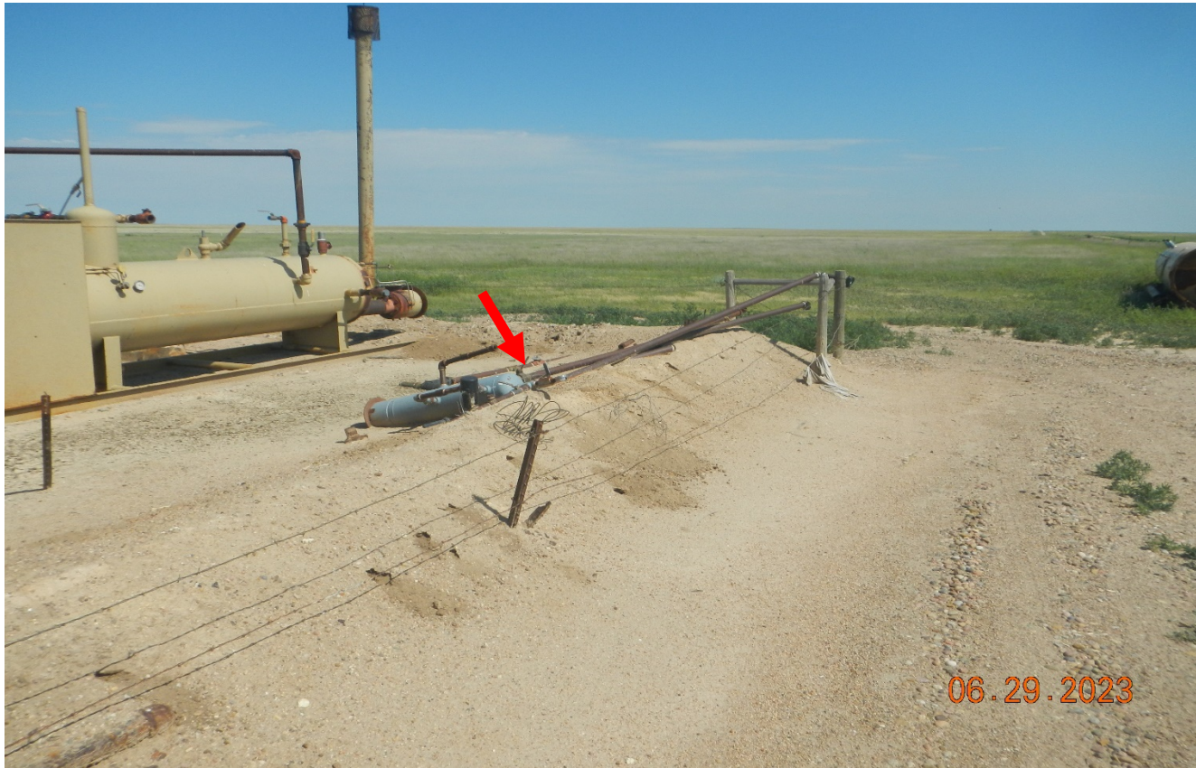
Photo 4. There is unused disconnected pipe that needs to be removed.
