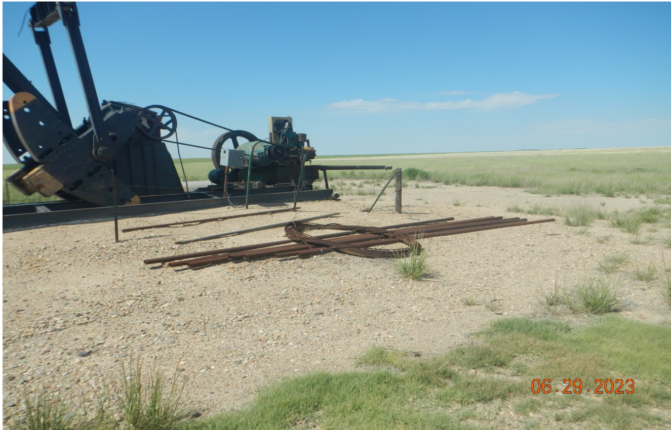
Photo 7. There is unused pipe and cable that need to be removed.
