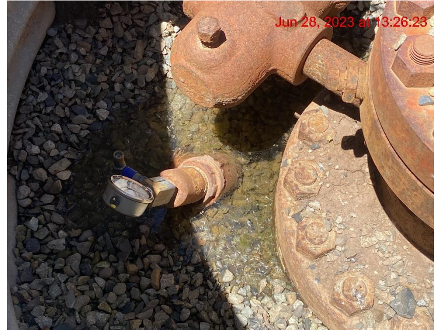
Unknown Fluid Accumulating Around Bradenhead – Photo #04922
