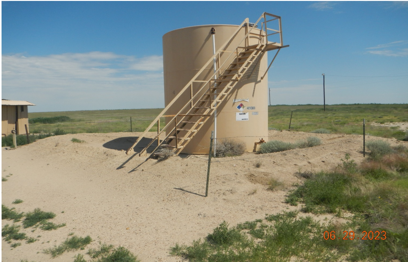
Photo 7. Facing at the north side of the location. The fence around the tank battery is inadequate to prevent livestock entry and is not maintained. Berm is insufficient to contain a spill (150% of tank capacity).
