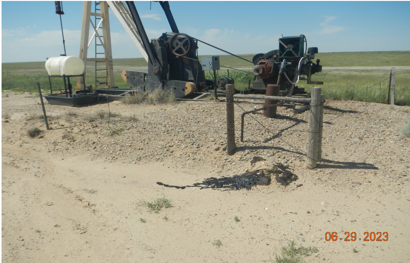
Photo 5. There is oily sludge that has spilt onto the ground that needs to be cleaned up.
