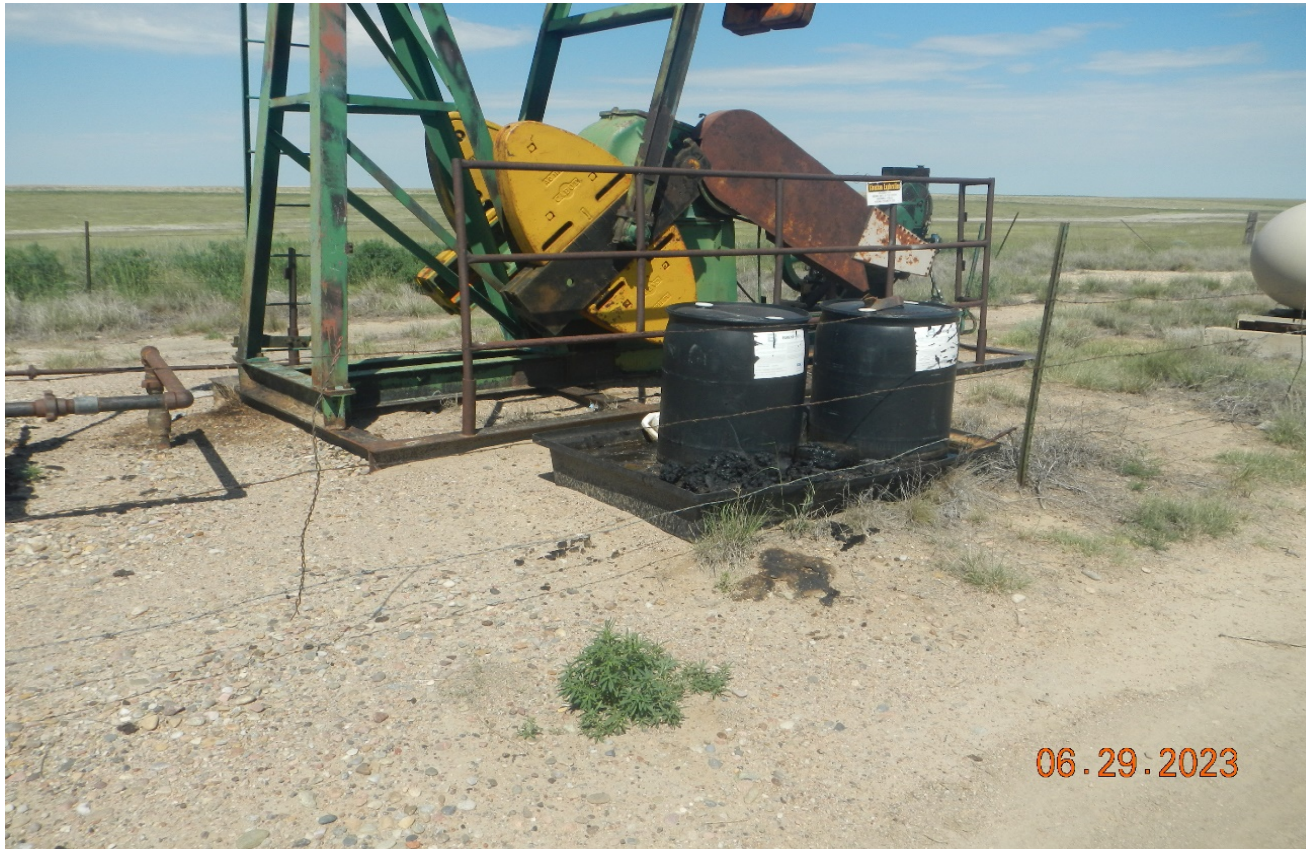
Photo 2. Facing toward the pumpjack. There are two barrel stored in containment with faded labeling.
