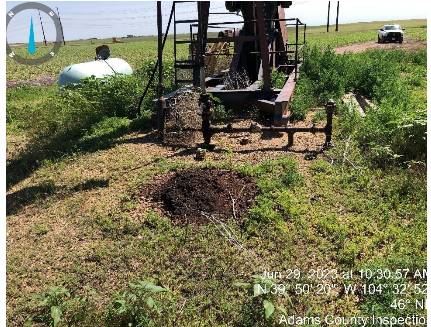
Photo# 2 Stained soil in front of well head.
