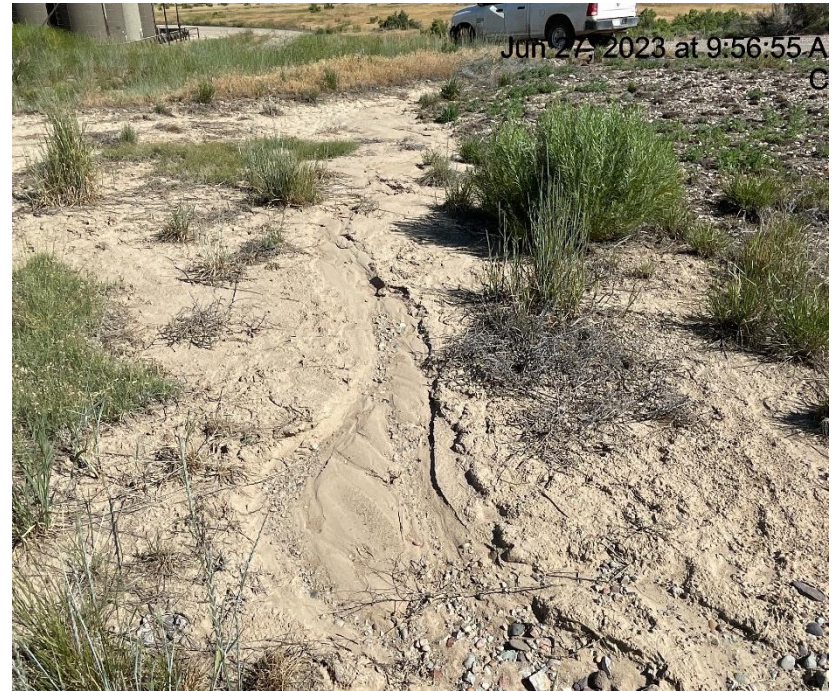
Photo # 1995 Erosion & transport of sediment off location/sediment choking of vegetation
