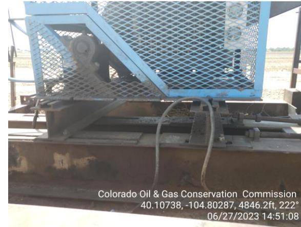
**Photo 14 stained soil in the pump jack frame under gas engine.**
