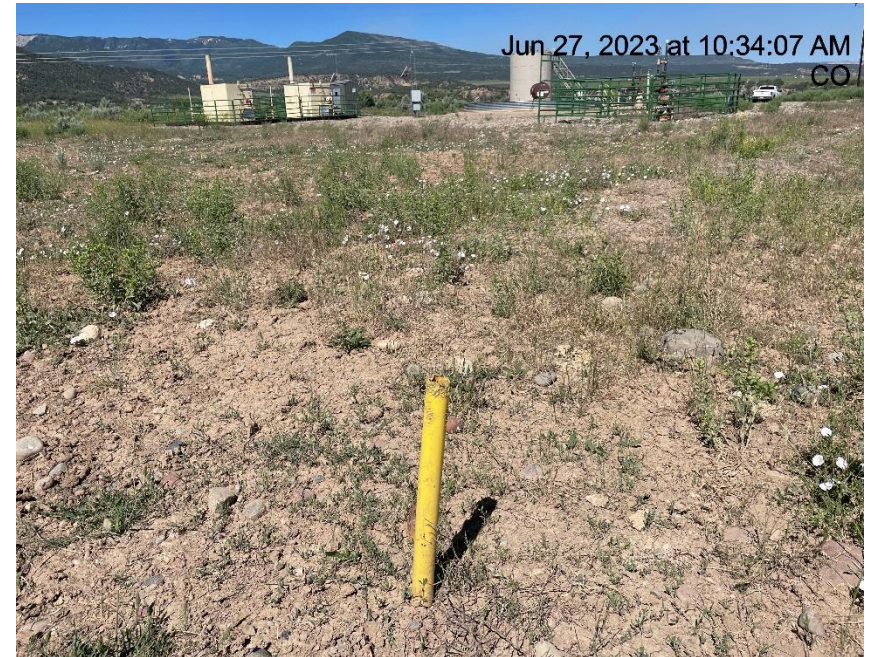
Photo # 2032 Improperly marked deadman
