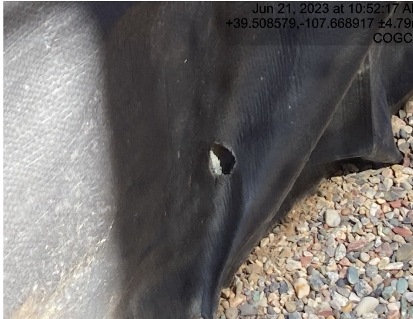
Holes in containment
