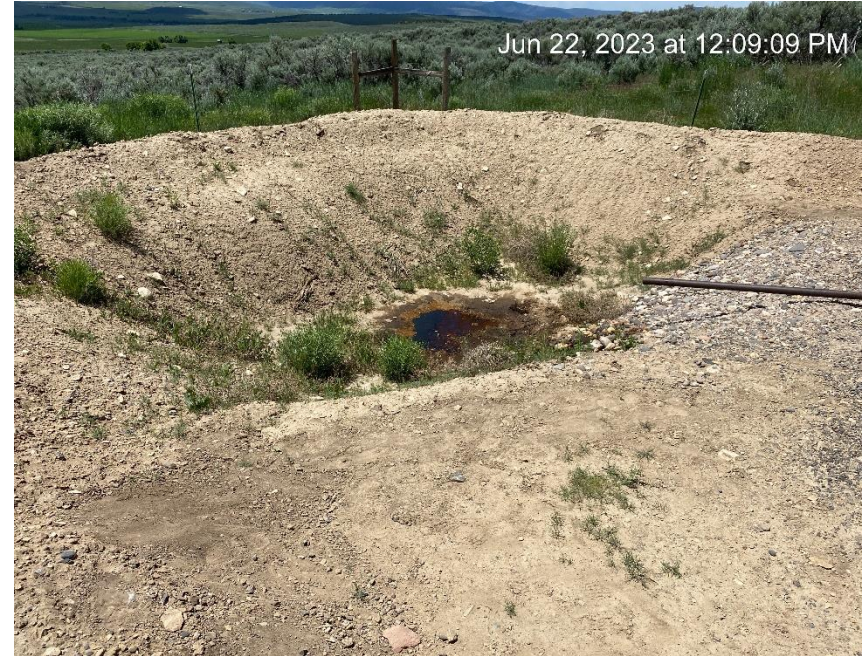
No Pit ID. Oil in pit. Open end line from tank.
