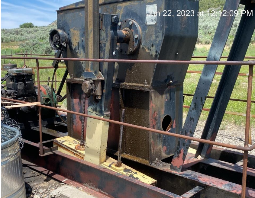
Engine and pumping unit oil leaks
