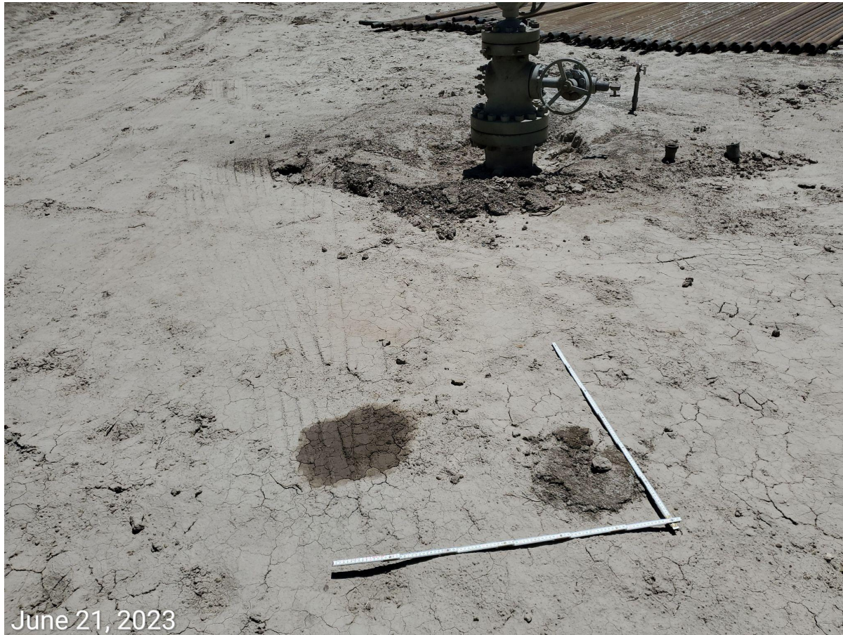
Photo 7: Photo shows stained soils due to new/recent spills.
