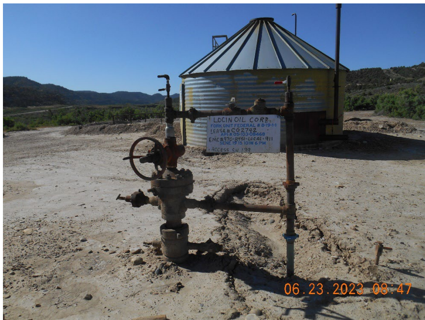
Injection wellhead with sign
