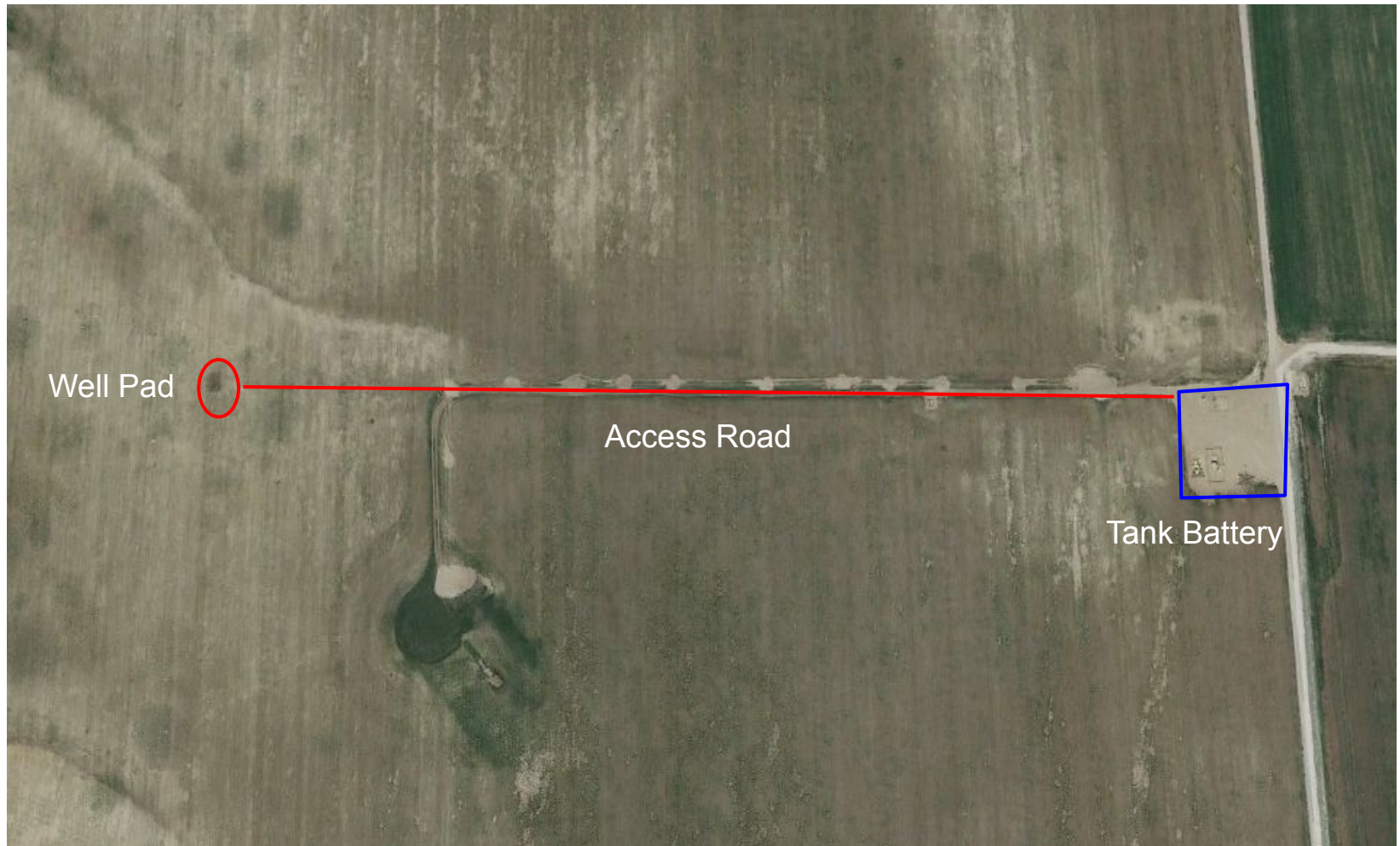
Photo 1. 2021 aerial imagery of the well pad and access road. Note: Tank battery highlighted in blue remains for the Edwards 43-9 well API #123-20867.
