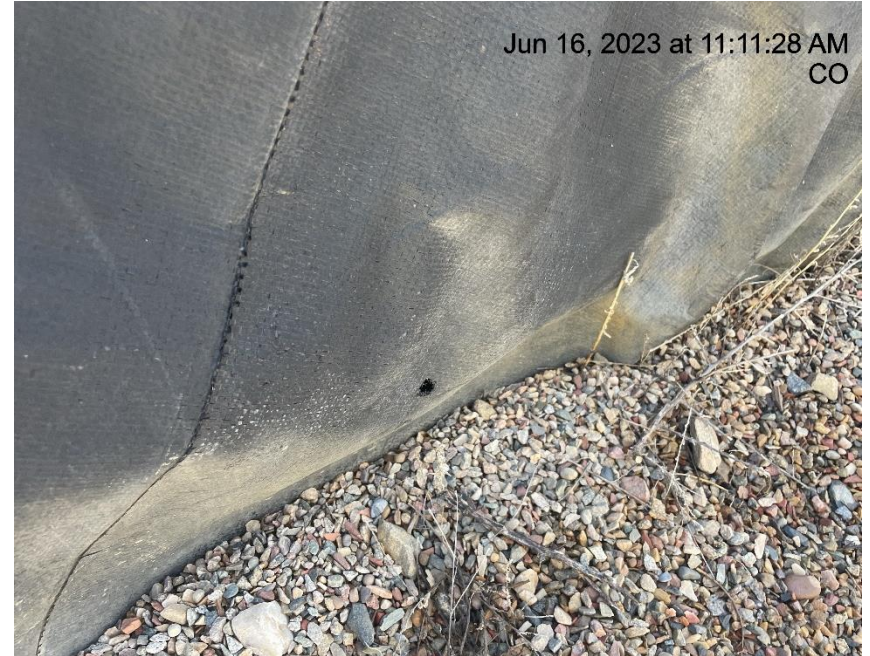
Photo # 848 Hole in containment line/liner needs maintenance
