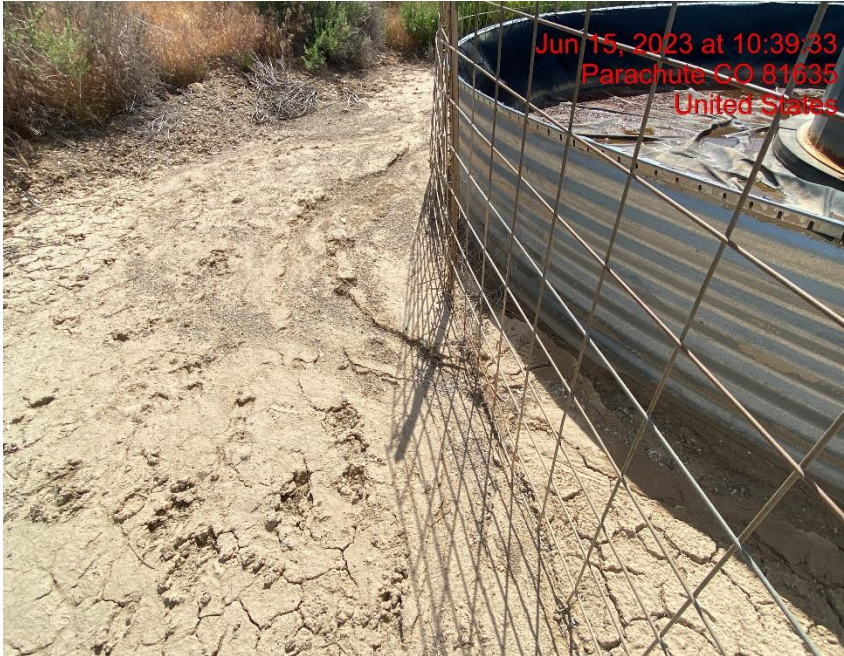
Rill Erosion Transporting Sediment onto Location – Photo #04494
