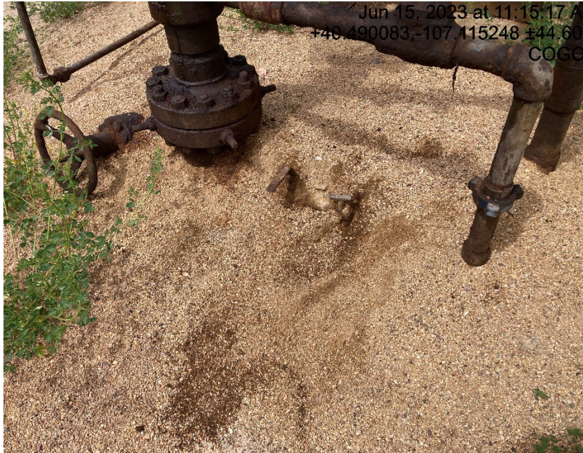
Staining and Braden head access. Stained soil under fresh gravel.
