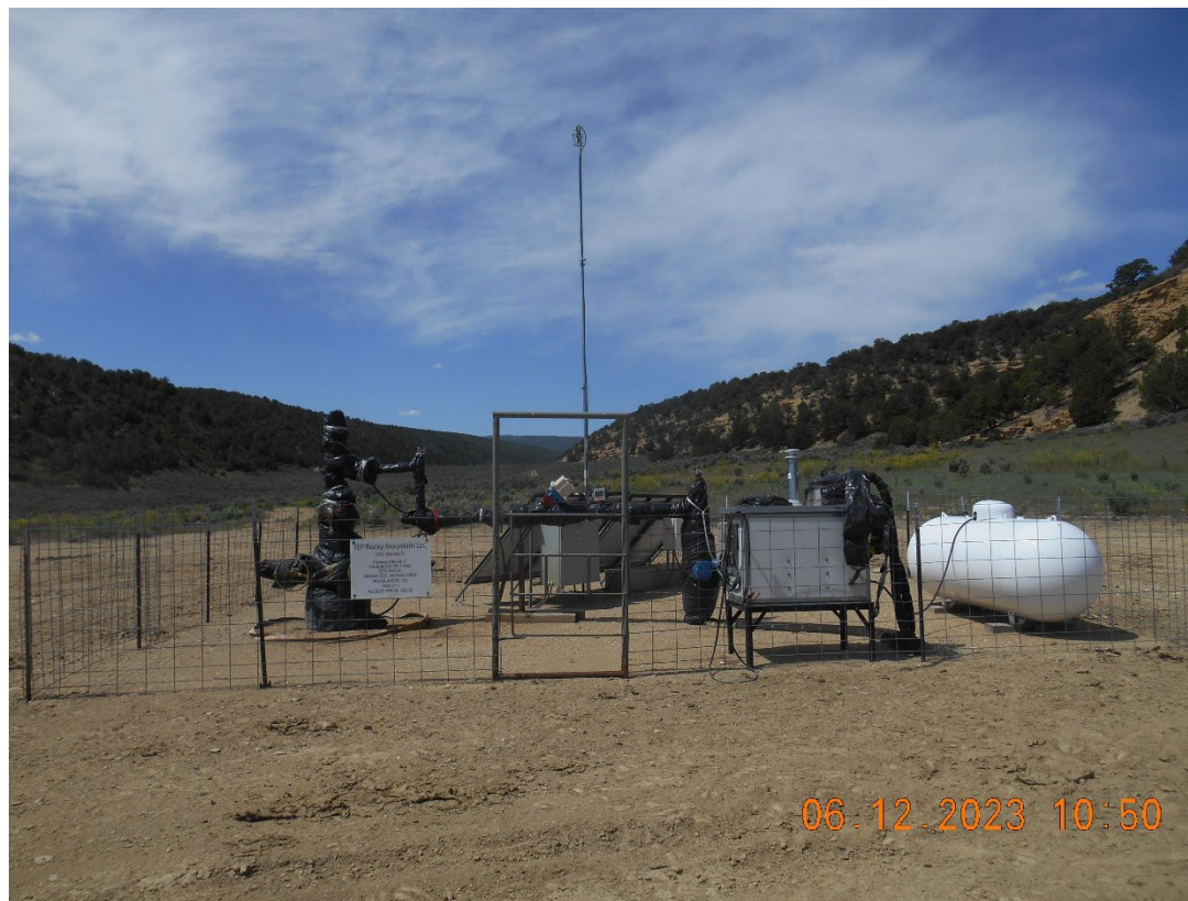
Injection wellhead & line heater
