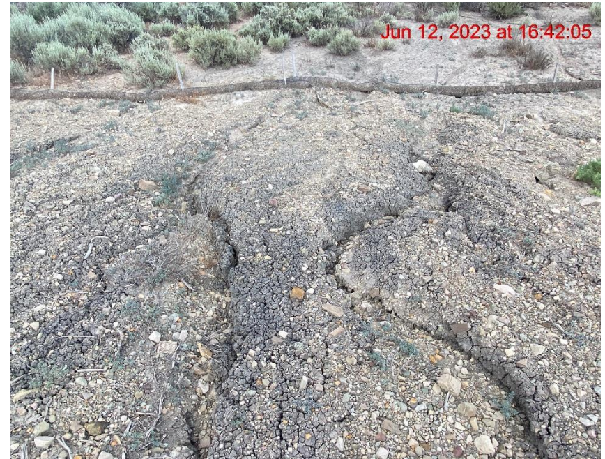
Rill Erosion Transporting Sediment Off-Location – Photo #04391
