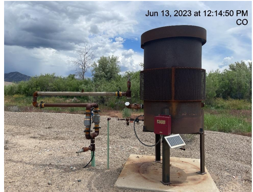
Photo # 348 Unused Equipment – ECD is disconnected & not operational
