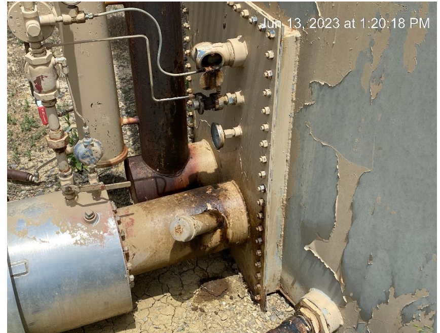
Leaking equipment and stained soil
