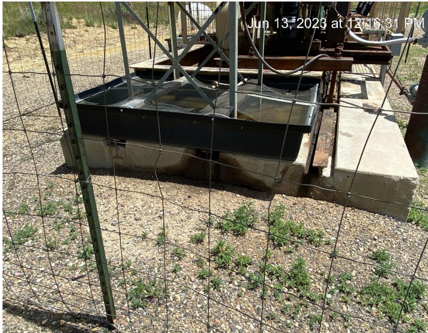
Leaking equipment and stained soil
