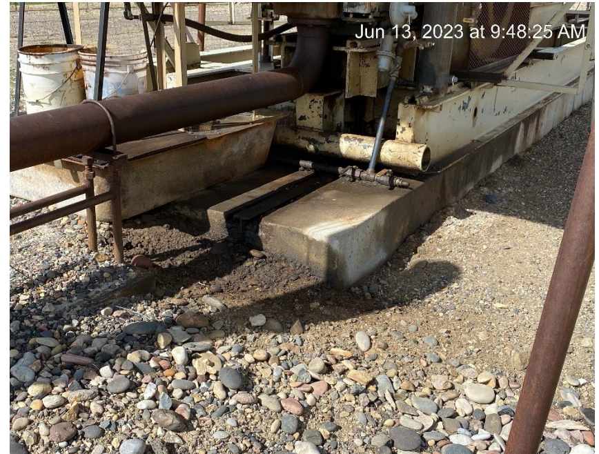
Equipment leaks and stained soil
