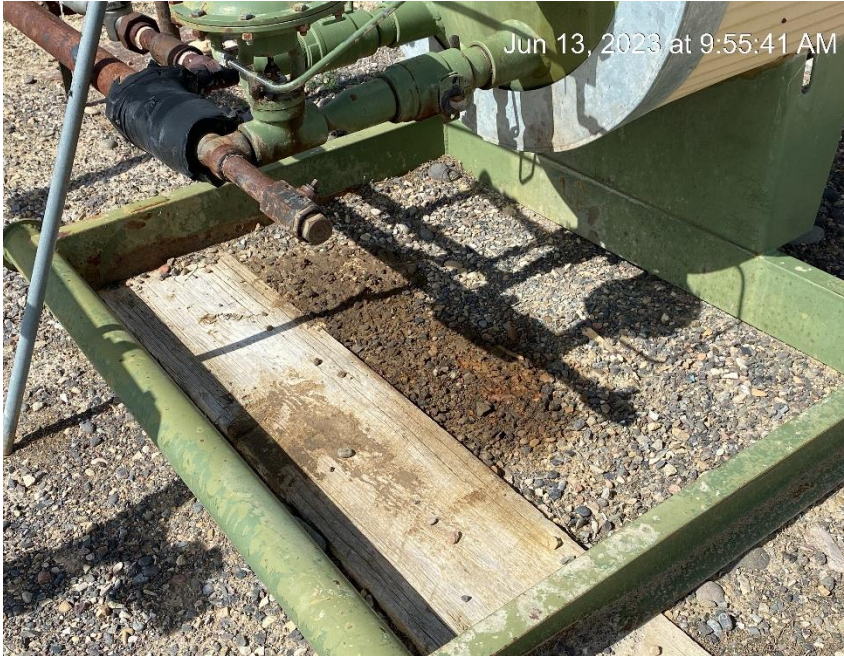
Stained soil from leaking equipment
