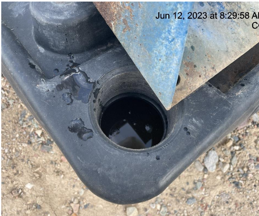
Photo # 60 Chemical containment full/Failure to maintain chemical BMP's
