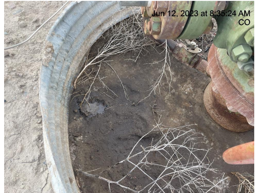
Photo # 71 Stained soils & gravel inside GUCCINI 41C wellhead cellar
