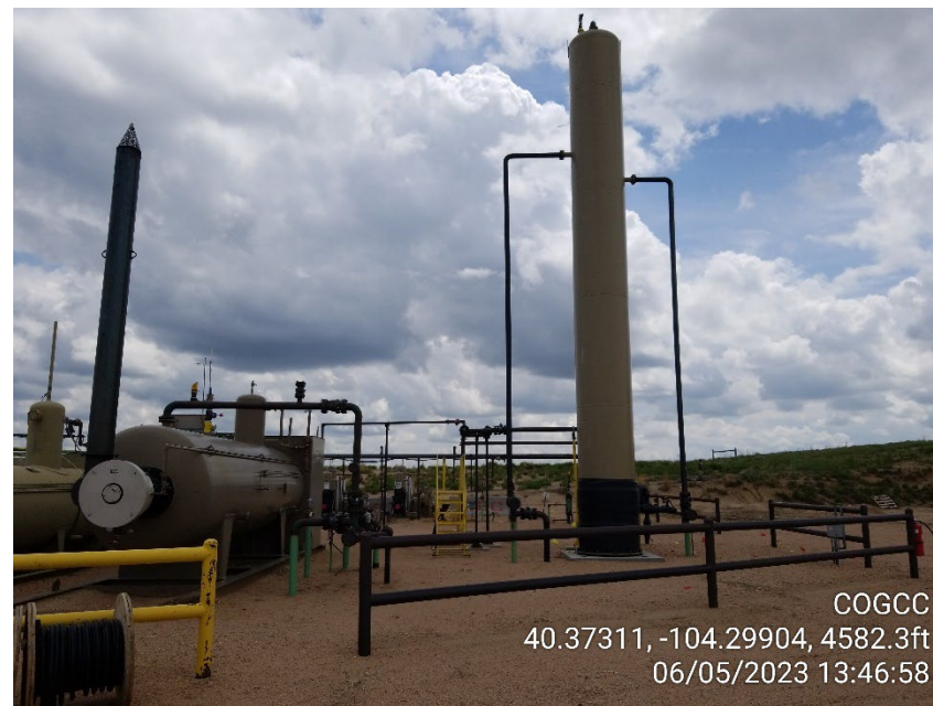
Photo 6 – Separator and VRT
