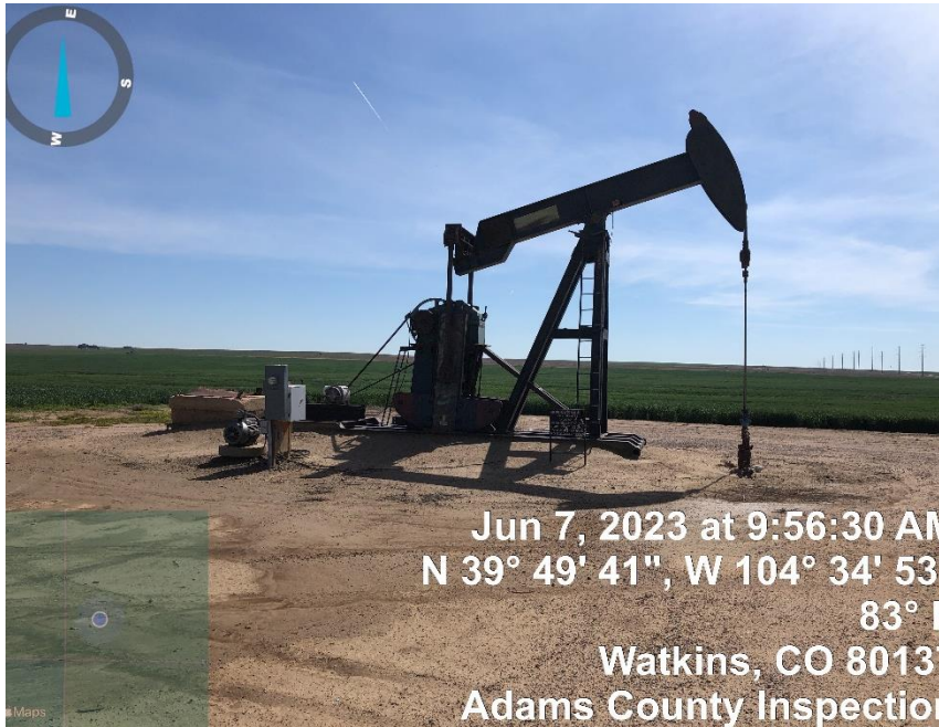
Photo#3 Pumpjack/Wellhead
