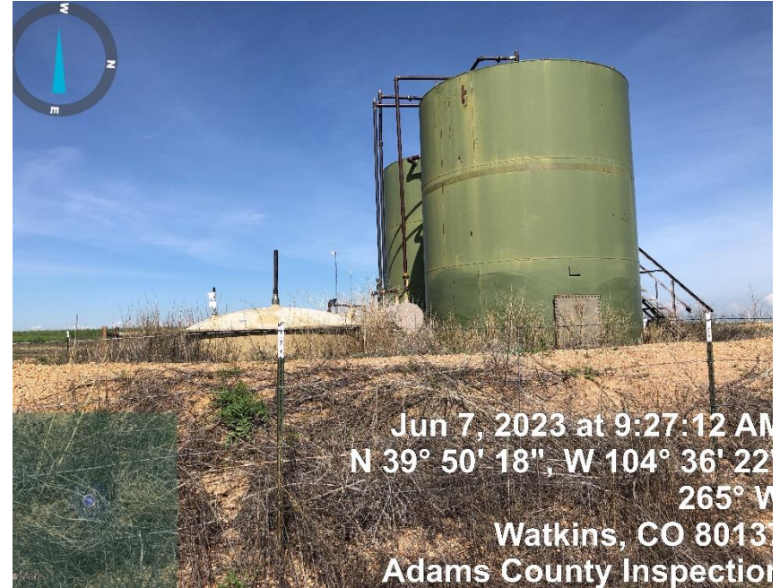
Photo#4 Produced Water Tank
