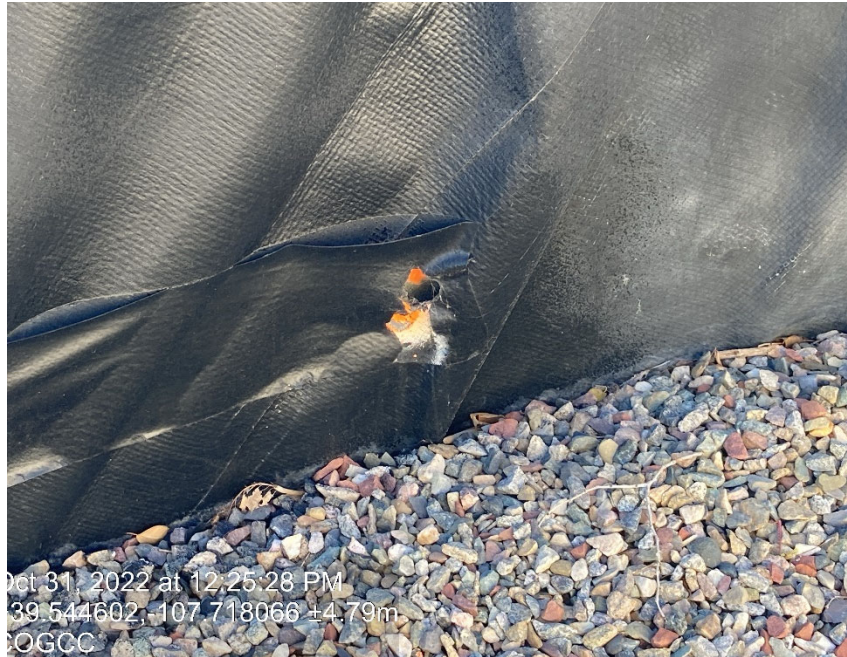
Previous inspection photo of holes in containment document # 700704664
