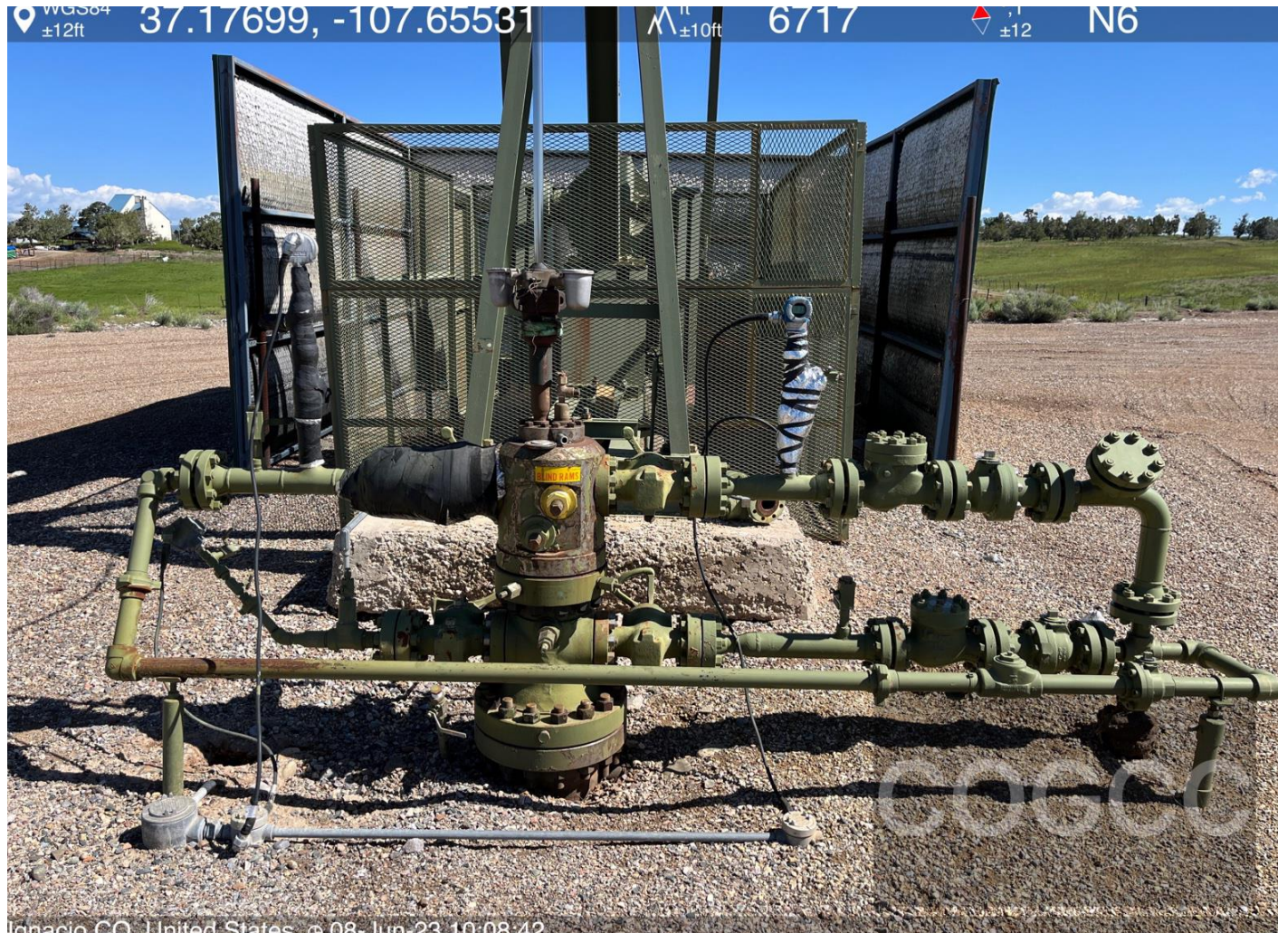
Photo #2. View of wellhead assembly.
