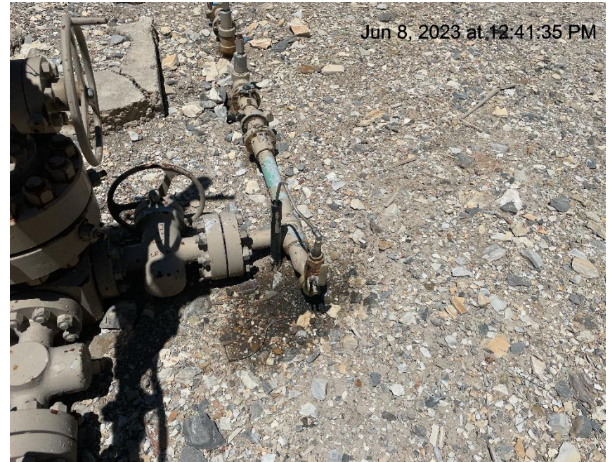
Photo # 9624 Line connected to wellhead leaking/stained soils & gravel
