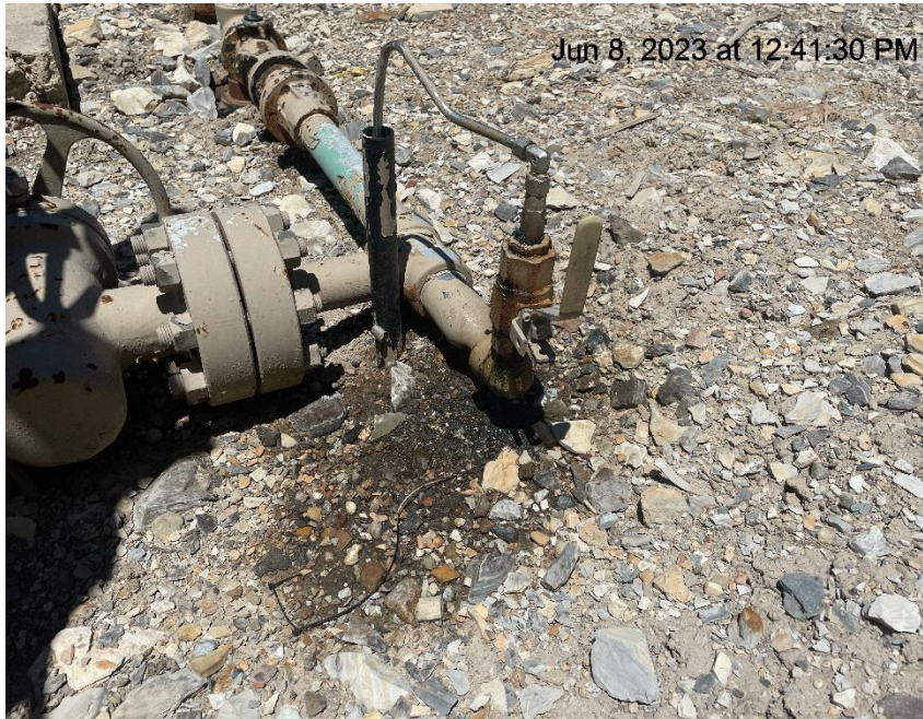
Photo # 9891 Line connected to wellhead leaking/stained soils & gravel
