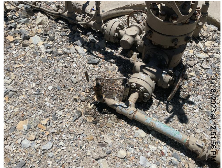
Photo # 9900 Line connected to wellhead leaking/stained soils & gravel
