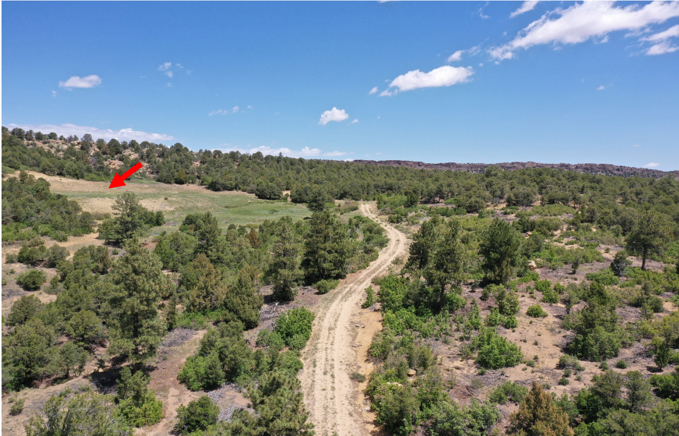
Photo 1. 2022 Drone aerial photo facing north along the former access road. The road was not recontoured and reclaimed but continues on past the location. Location shown at red arrow.
