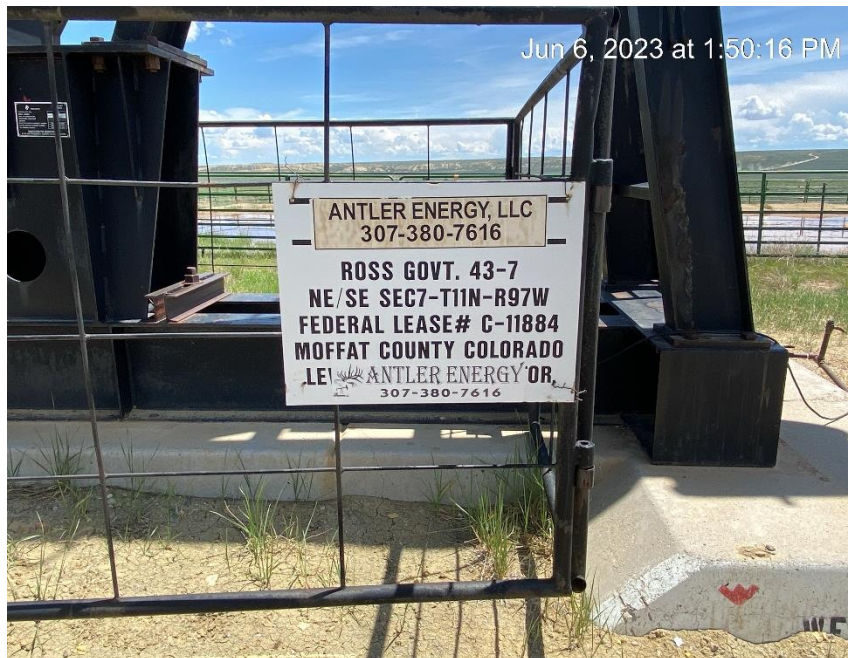
Sign at wellhead missing required information
