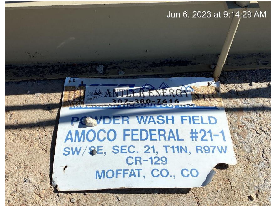
Wellhead sign on the ground. Missing required information.
